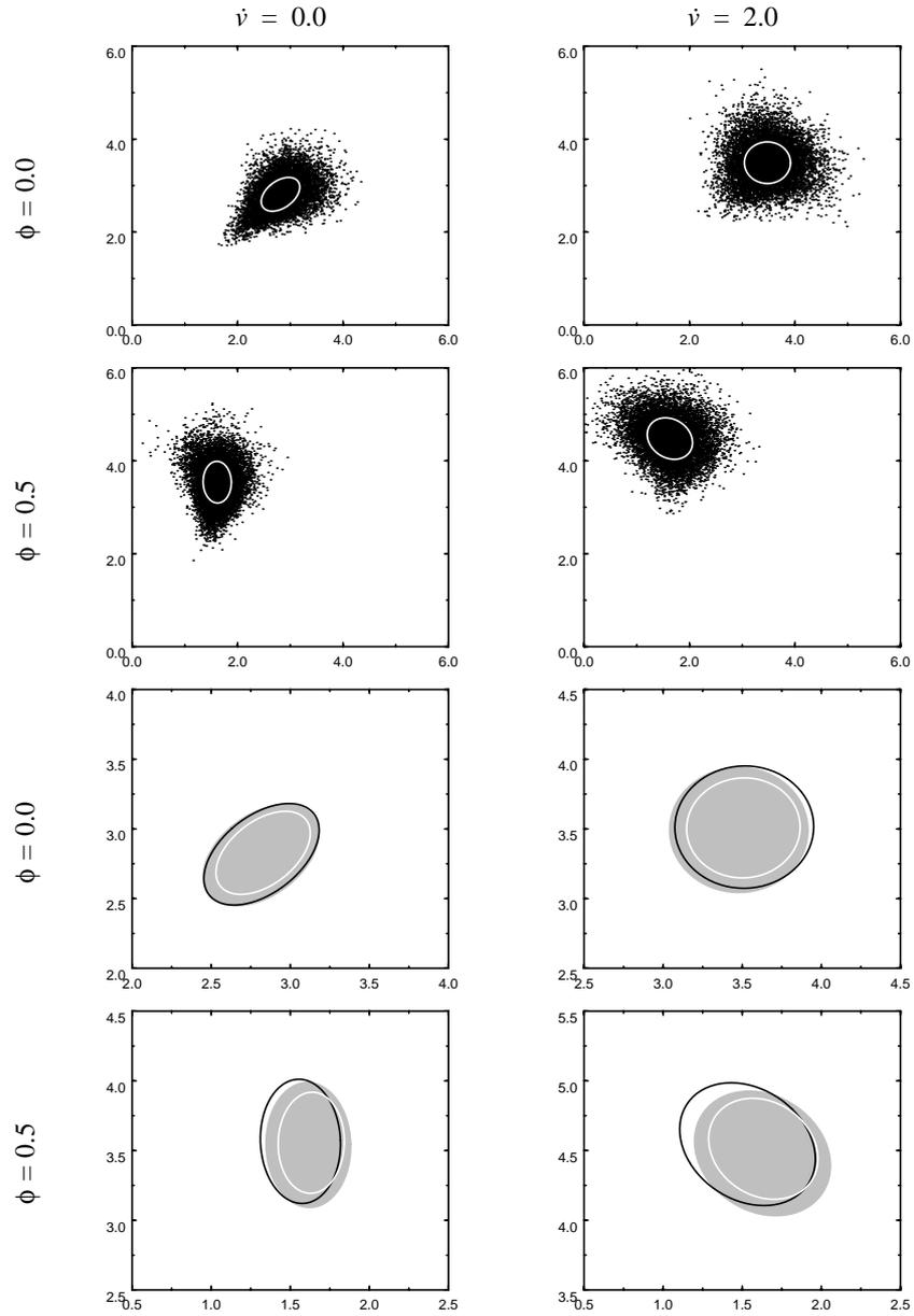
Figure 2 Top two rows: Monte Carlo trials of the kinematic model, projected onto the  $(x, y)$  plane (black dots). Initial conditions  $x=y=0$ ,  $\theta=\pi/4$ ,  $v=4ms^{-1}$  in all cases. Separate graphs for steering angle  $\phi=(0, 0.5)$  radians and acceleration  $\dot{v}=(0, 2.0) ms^{-2}$ . Best-fitting ellipse at  $1sd$  shown in white. Bottom two rows: Same conditions, best fitting ellipses (grey) with covariance estimated by EKF (white) and the CUF (black). NB: change of scales.
