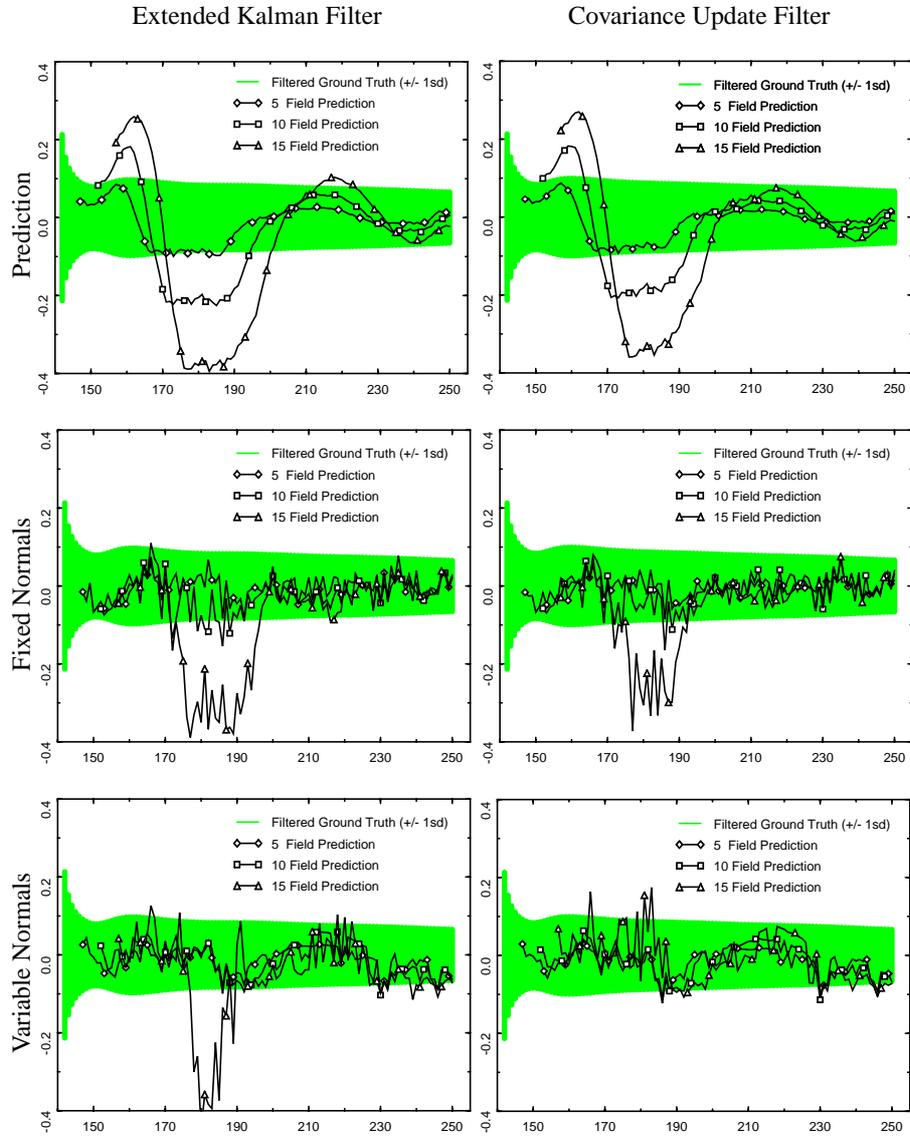
Figure 4 Performance of the kinematic model using the EKF estimator (left); and the CUF estimator (right). “Ground truth” is given by ordinate = 0.0 (scaled in metres), and  $\pm 1$  sd. of the estimated y-parameter is shown shaded.
