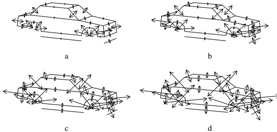
Figure 3 Search regions (perpendicular in the image to the projected model lines) determined by  $\pm 3$  sd of the estimated filter covariance for forward predictions of (a,b,c,d) 0, 5, 10 and 15 fields (@ 50 Hz).
