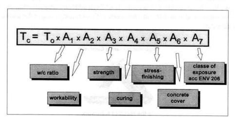
As can be seen, the durability, or life time of a structure is not only a question of w/c ratio and workability but the formula shows clearly the influence of this two factors. Tables 10 and 11 give some more details about the two factors.
