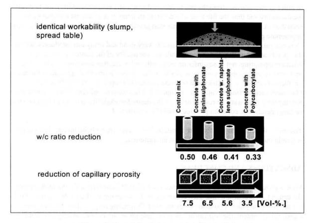
Figure 2. Correlation between w/c and porosity
