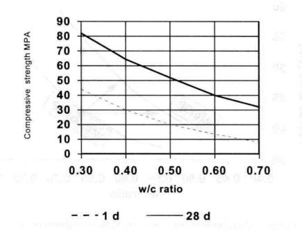
Figure 3. Correlation between w/c and compressive strength
