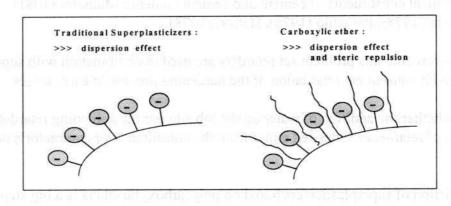
Figure 5. Mechanism of action of superplasticizers molecules
