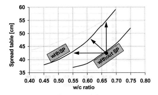
Figure 4. Correlation between w/c/ ratio and workability of concrete (SP = Superplasticizer)
