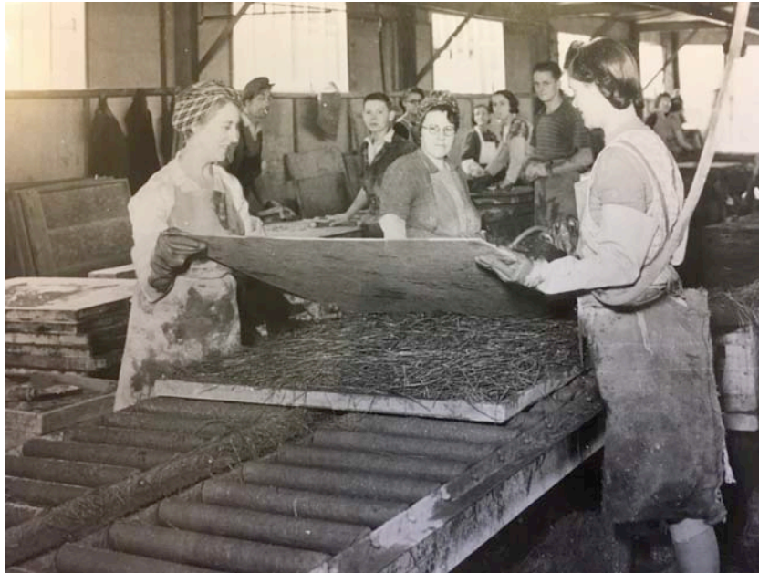
Figure 5.10 Women war workers at the En-Tout-Cas Factory manufacturing the Seco Hut panels. (Photo courtesy of Paul Francis, Airfield Research Group)
