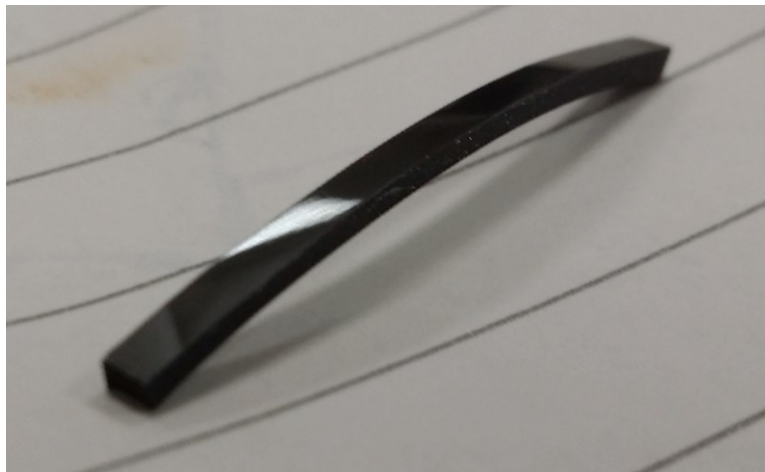
Figure 96. A SiC test bar showing the arching effect, likely due to drying too fast.
