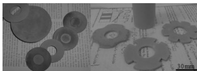
Figure 10. \text{Si}_3\text{N}_4 objects fabricated by means of LOM. Reprinted with permission from [26].
