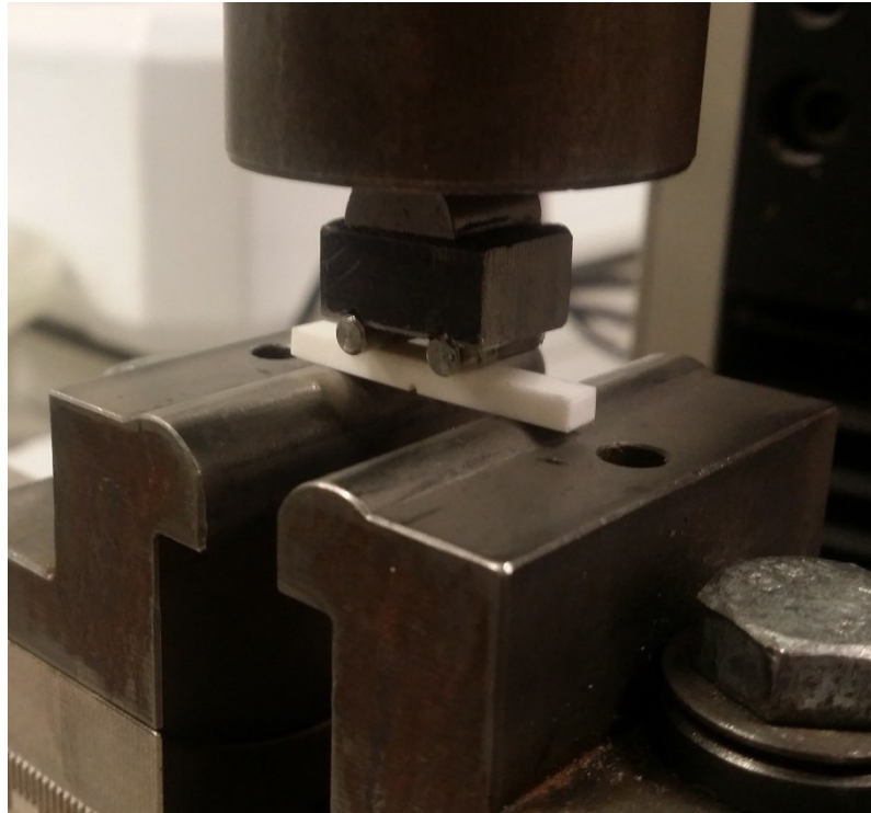
Figure 38. A composite sample with a sharpened notch being measured in 4 point bending.
