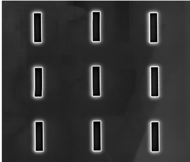
Figure 111. An array of trenches milled into a silicon substrate.
