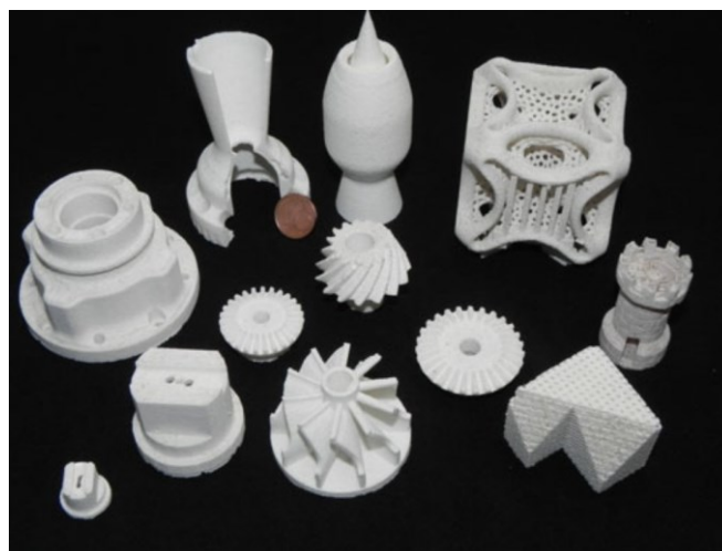
Figure 6. Al_2O_3 parts produced by SLM. Reproduced with permission from [16].
