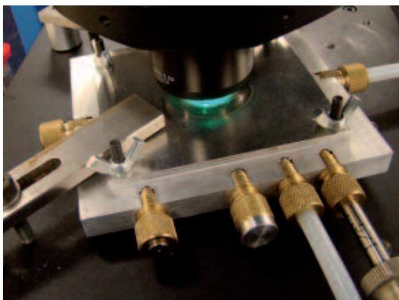
Fig. 1. Successful application of a newly developed flow cell with inert sliding injector for study of interaction of levitated particles with the initiators of atmospheric oxidation  $\text{NO}_3$  and  $\text{N}_2\text{O}_5$ . Additional ports allow horizontal visualisation (e.g. using a borescope).
