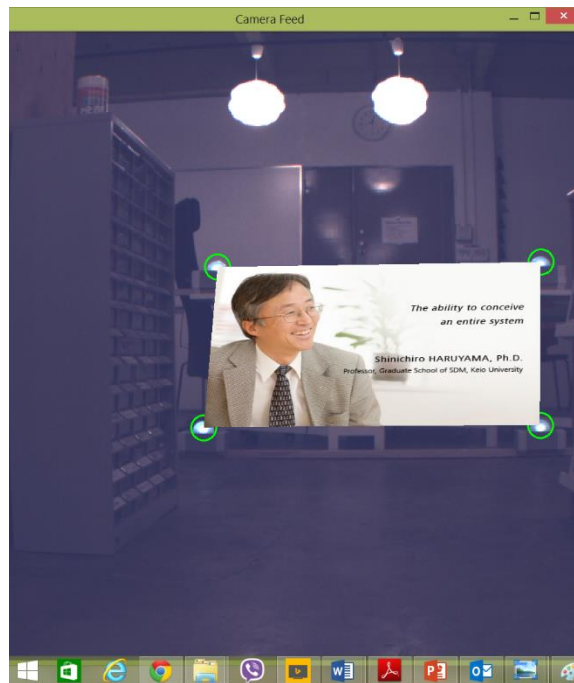
Figure 33: Finally virtual information is superimposed over real environment at the points computed earlier
