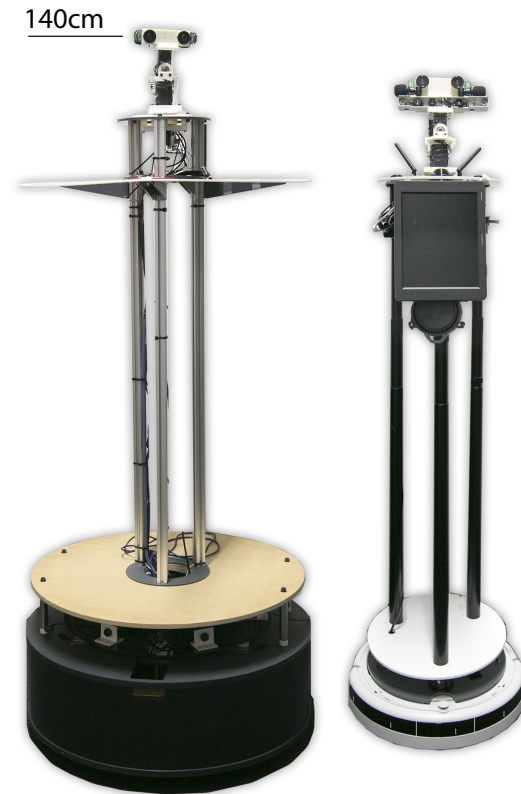
Figure 3.8: The two implemented versions using Omni Wheel and Roomba
