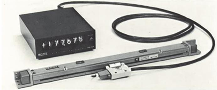
(a) Flux response type magnetic scale
