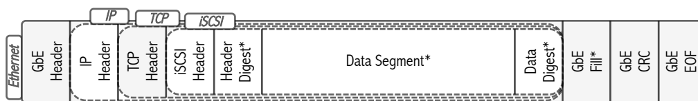
Figure 2.5: Layers of iSCSI packet. The formation of the packet begins with data segment, creation of header and data digests, and an appropriate iSCSI header. Then, the packet is build out through TCP, IP and Gigabit Ethernet layers. (Optional fields are marked with *.)
