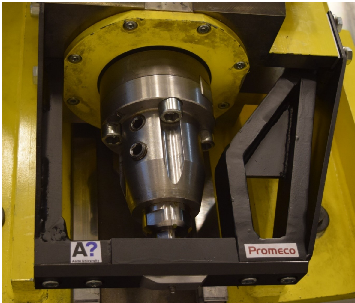
Figure 47 – The SSFSW tool module assembled on Aalto University’s ESAB Legio FSW machine
