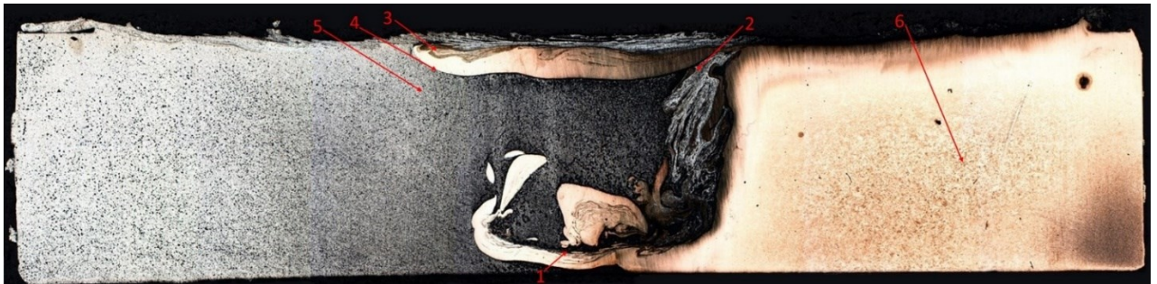
Figure 65 – Optical macrograph of the optimized weld, areas of interest detailed by Figure 66 are marked from 1 to 6
