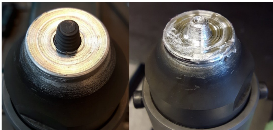
Figure 49 – An unused probe and clean shoulder vs. shoulder and probe filled with sticky Al
