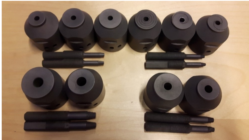
Figure 40 – Manufactured conventional FSW shoulders and probes
