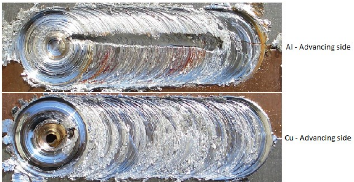
Figure 18 – Effects of material positioning (adapted from Liu et al. [37])
