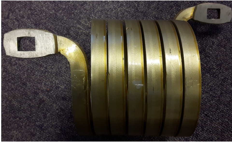
Figure 21 – Conventional monolithic Al bus bar
