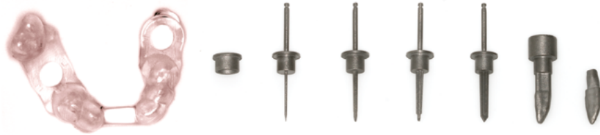
Figure 1. The 3D printed surgical tooling and implant, from left to right: guided template, sleeve, 4 drills, osteotome and one piece implant.
