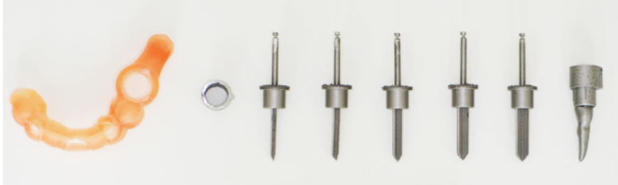
Figure 3. The 3D printed surgical tooling for cadaver No. 1. From left to right: guided template, sleeve, 5 drills and osteotome.
