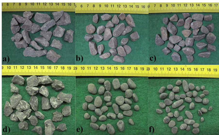
Fig. 3 The grains after 0 (a, d), after 60,000 (b, e), and 120,000 rotations (c, f), respectively. Top row displays andesite from Recsk (images: a, b, c); bottom row shows andesite from Nógrádkövesd: (images: d, e, f)
