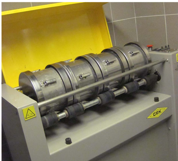
Fig. 2 The Micro-Deval test equipment with four drums
