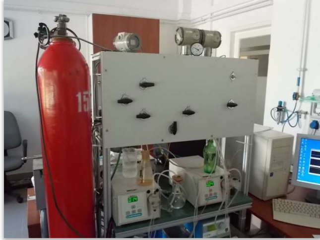
Figure 5. Hydrate forming test-equipment
