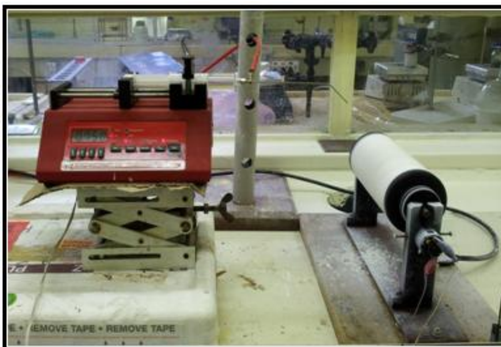
Figure 3.1. Electrospinning set-up for fabrication of nylon 6 composite nanofibers
