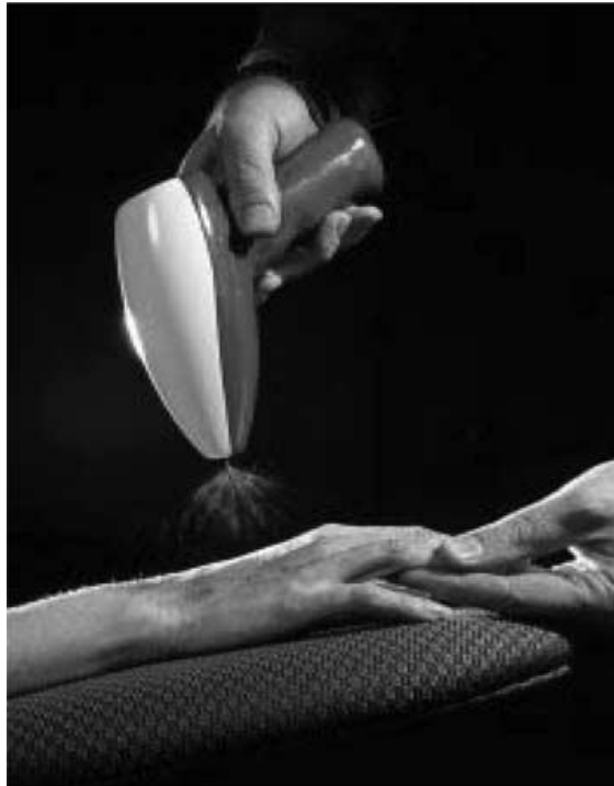
Figure 2.19. A hand-held electrospinning devices for wound dressing 167
