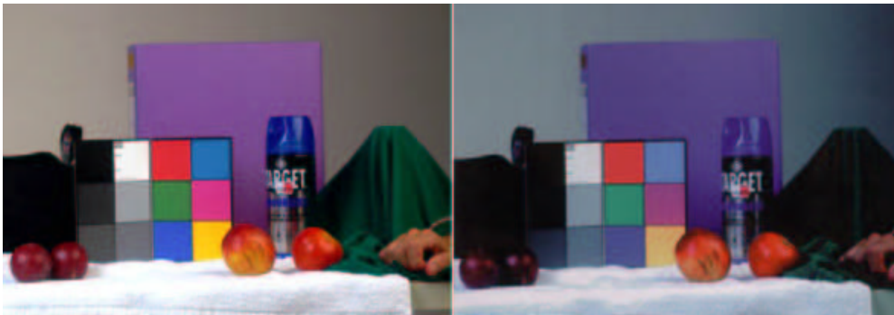
Figure 35. Comparison of original image (L) and copy of thermal inkjet print (R). (Giloi, 1999)
