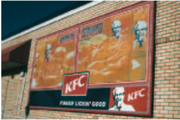
Figure 8. Photograph of the discoloration caused by ink leaching out of a thermal inkjet poster. (Giloi, 1999)
