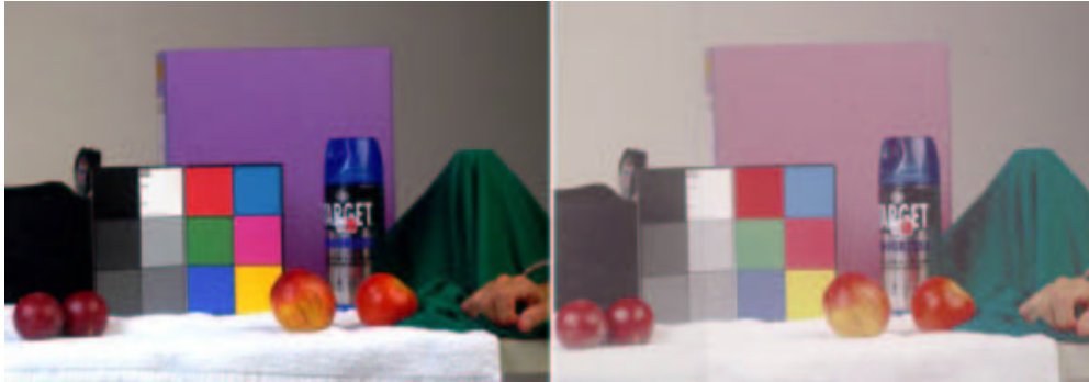
Figure 37. Comparison of original image (L) and copy of continuous flow inkjet print (R). (Giloï, 1999)
