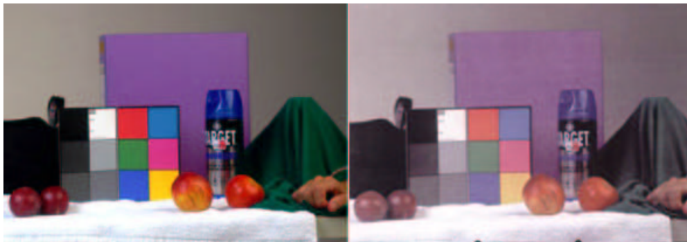
Figure 43. Comparison of original image (L) and copy of colour laser print (R). (Giloi, 1999)
