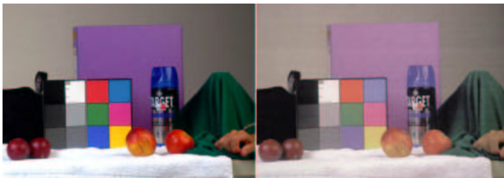
Figure 45. Comparison of original image (L) and copy of electrostatic print (R). (Giloi, 1999)
