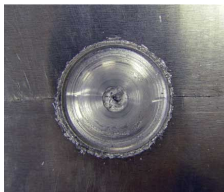
Figure 5.8: First Static weld.
