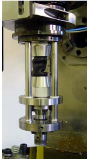
Figure 5.11: Tool after static weld test.
