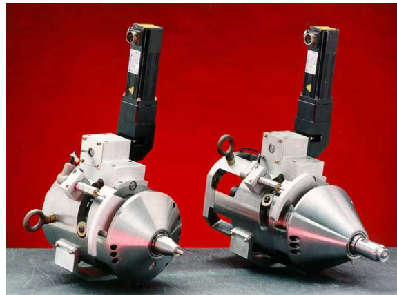
Figure 3.8: NASA's retractable pin tool.
