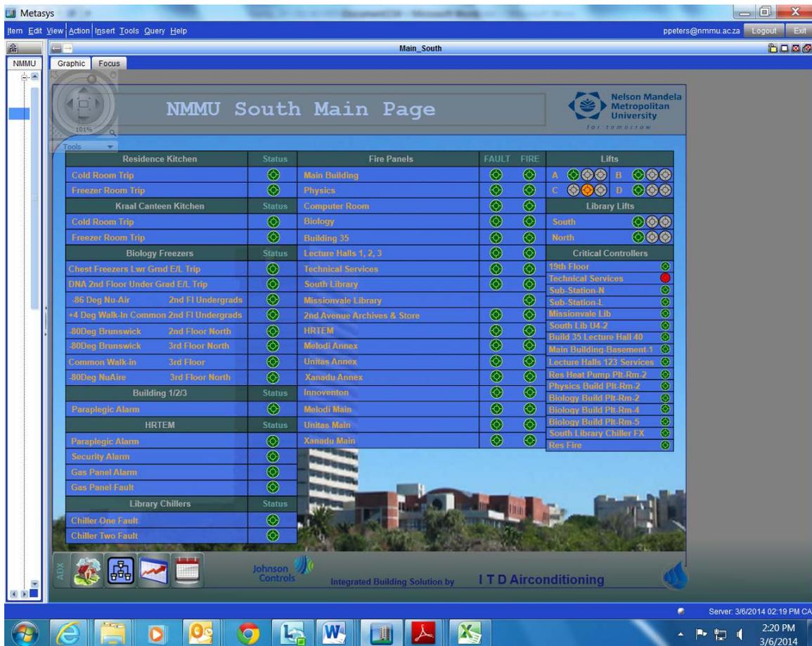
Figure 4.6: NMMU South Campus Air Conditioning Main Page for JCBMS
