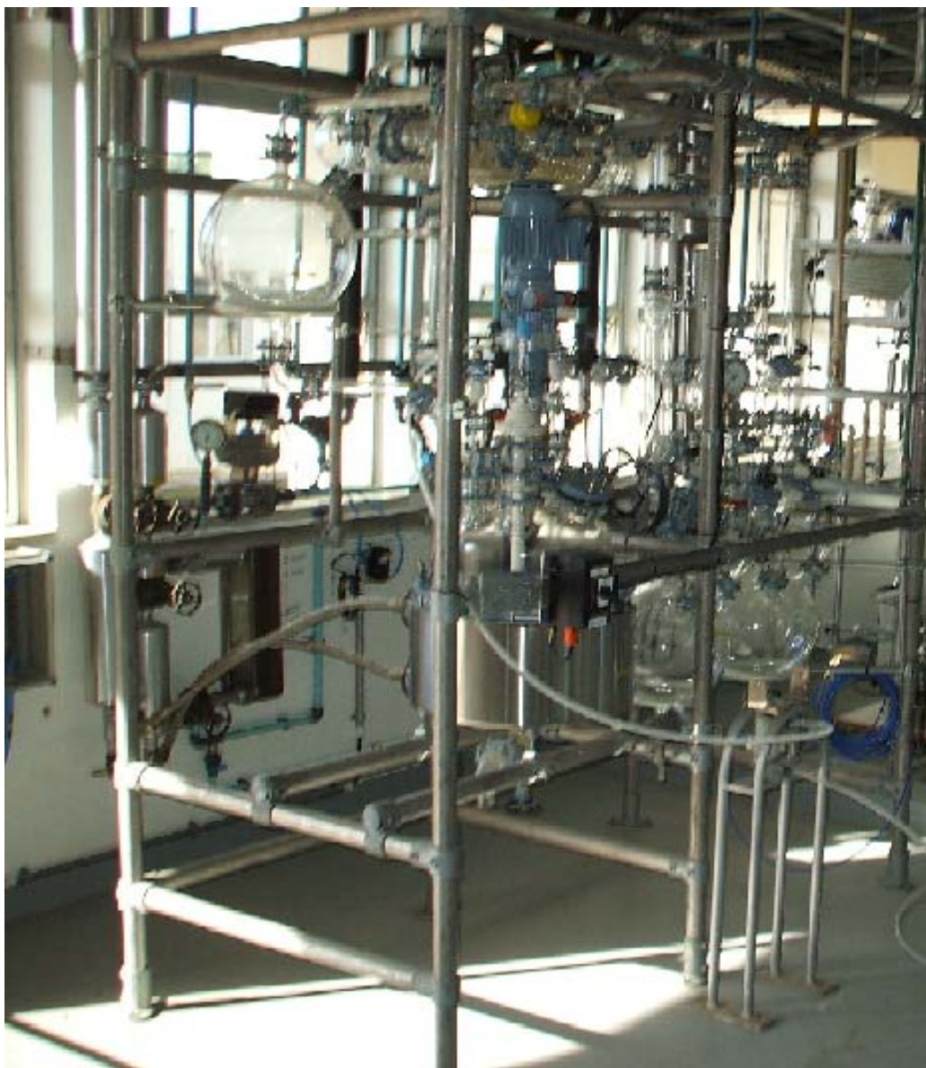
Figure 2.2: 30L Büchi Chemreactor system
