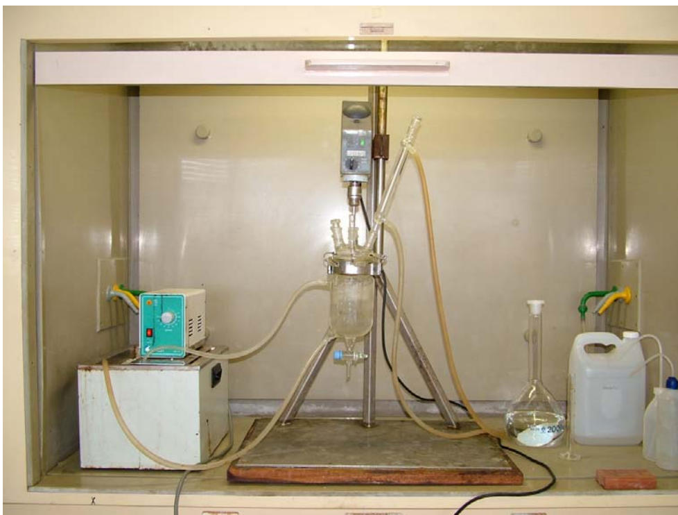
Figure 2.1: Double-walled glass reactor, equipped with overhead stirrer and connected to heater circulator bath
