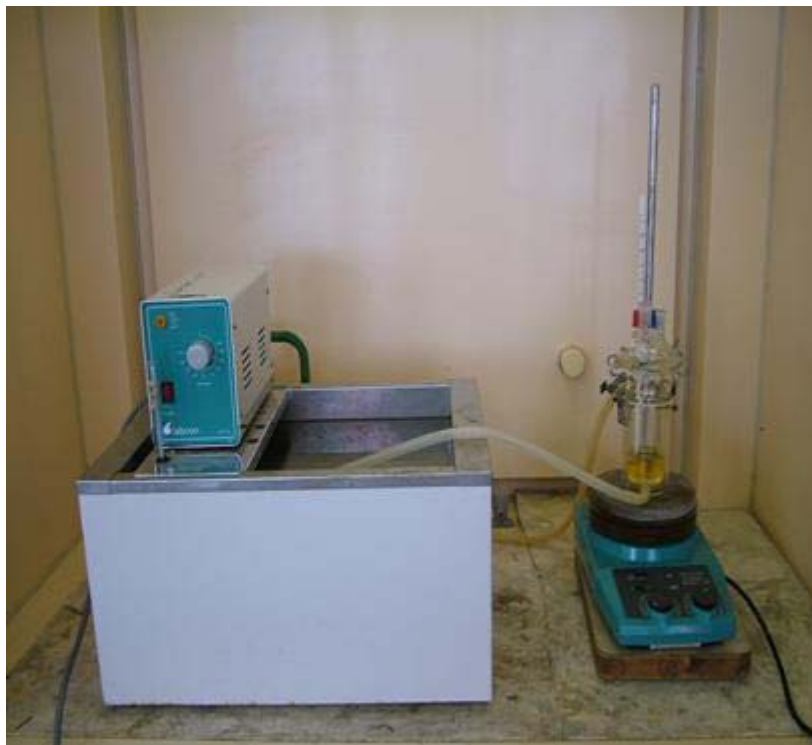
Figure 2.4: Direct electrochemical oxidation setup
