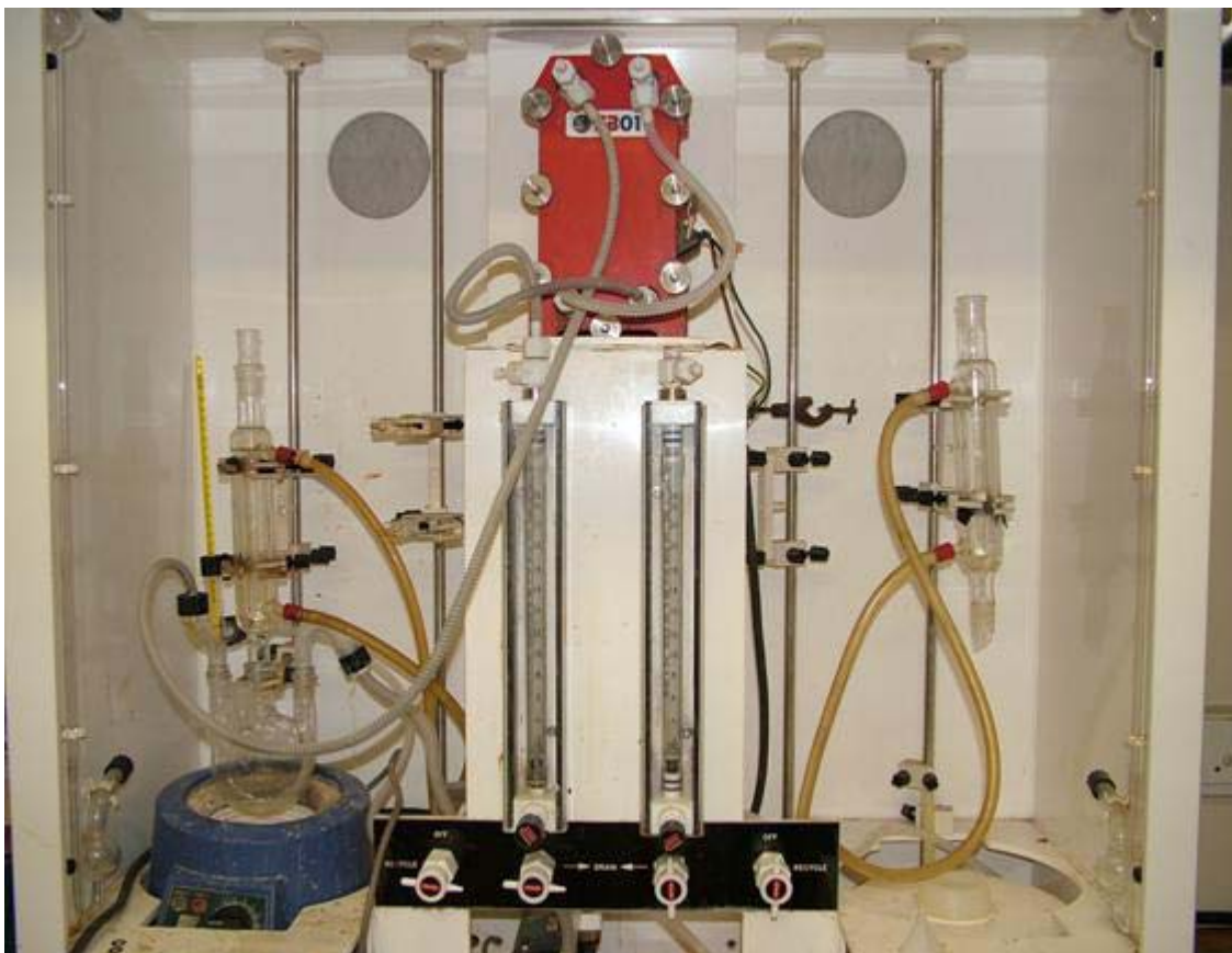
Figure 2.3: Batch recirculation flow cell for scale-up
