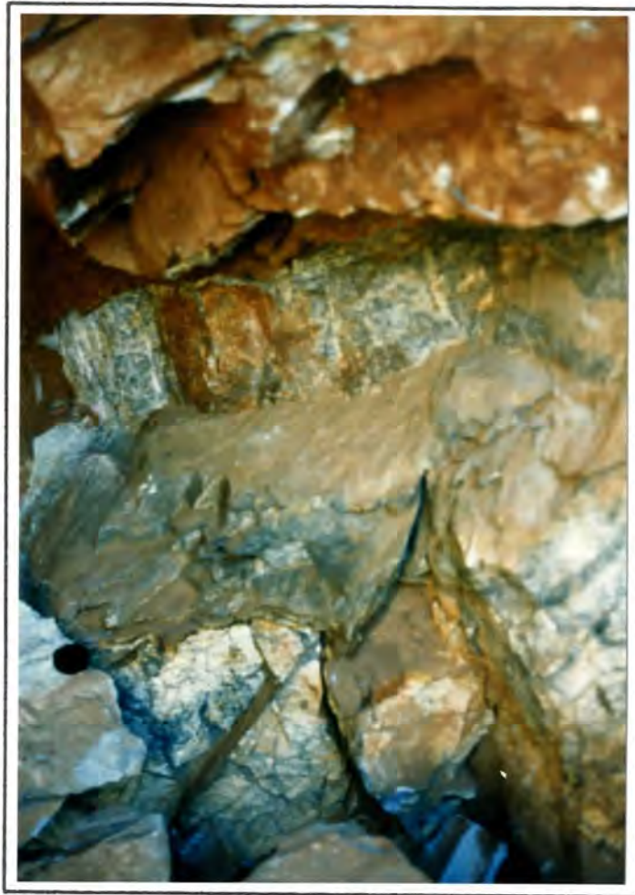
Plate 3.10. The Quartz Vein Reef exposed in old workings of the Zandrivier Mine. The reef is about 30cm thick. Note the brecciated chert which occurs just below the reef.
