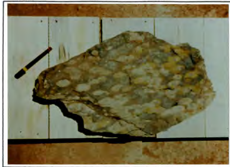
Plate 2.10. Sample of pillow basalt to show the ocelli used as markers in the strain analysis of the Mount Mare range. (Photograph courtesy of Maarten de Wit.)
