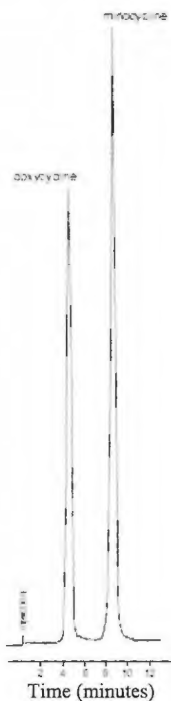
Figure 2.3. Typical chromatogram of the separation of minocycline (4.1 min) and doxycycline (8.1 min) in mobile phase
