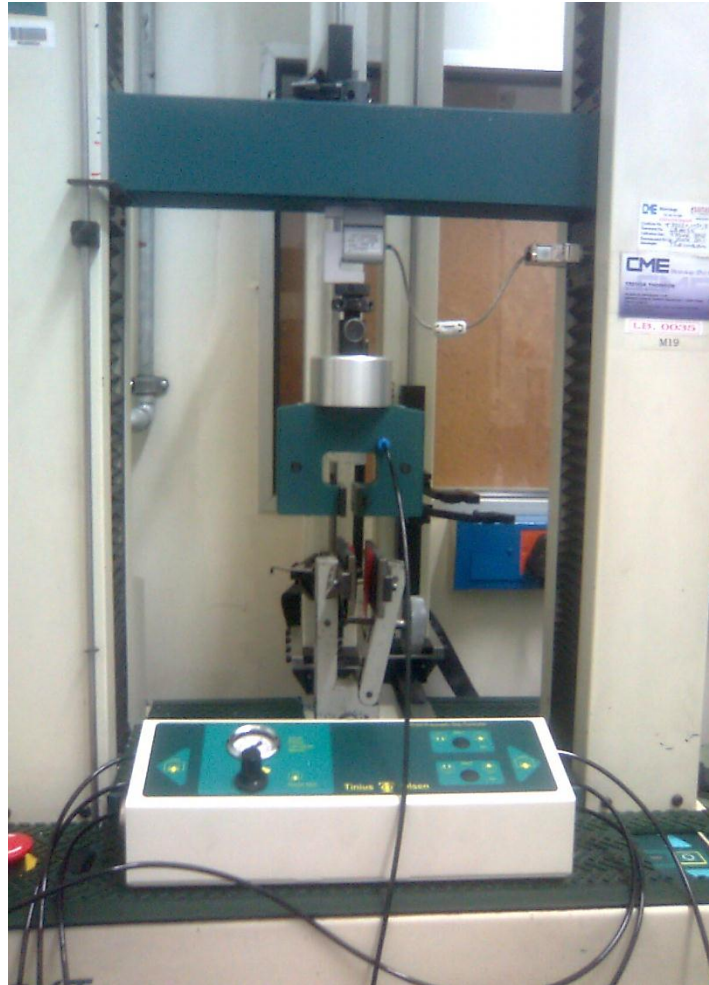
Figure 4.6 A full image of the Hounsfield tensometer H25KT used in the current study for the measurement of friction. The tensometer is housed at Aberdare Cables, Stanford, Port Elizabeth, South Africa.
