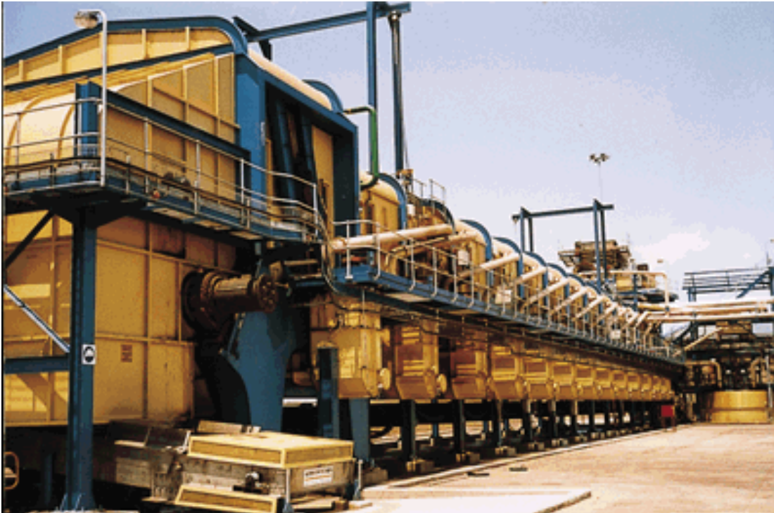
Figure 1.14: Counter current diffuser used by Tongaat Hullet S.A in the processing of sugar cane. ©Hullet S.A. 2004
