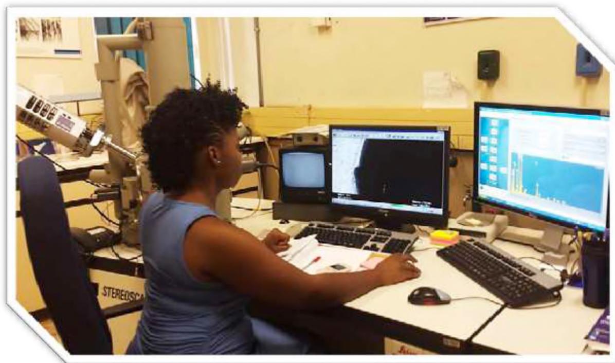
Figure 3.3: Leica Stereoscan 440 SEM linked to an OXFORD INCA EDS. The system consists of digital scanning electron microscope and three major subsystems the Fisons Keyex energy dispersive X-ray analysis system, the Finson LT7400 Cryo Transfer System and the Oxford Monochromator Cathodoluminescent system.
