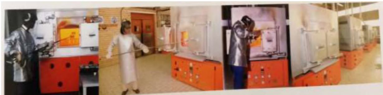
Figure 3.6: Fire assay-high temperature laboratory furnaces.
