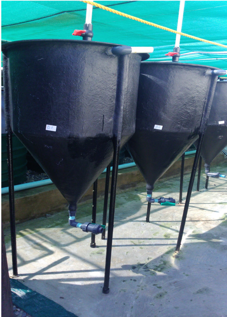
Figure 2.2. Settlement tanks (modified Guelph system) were connected to the recirculating system.
