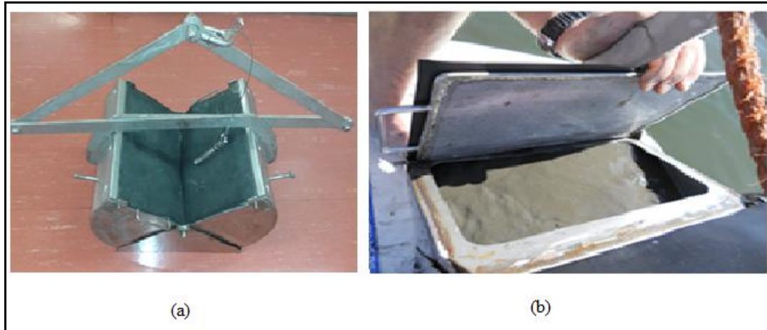
Figure 3.10: Picture of grab sampler used (a) and sampler containing sediment sample (b).
