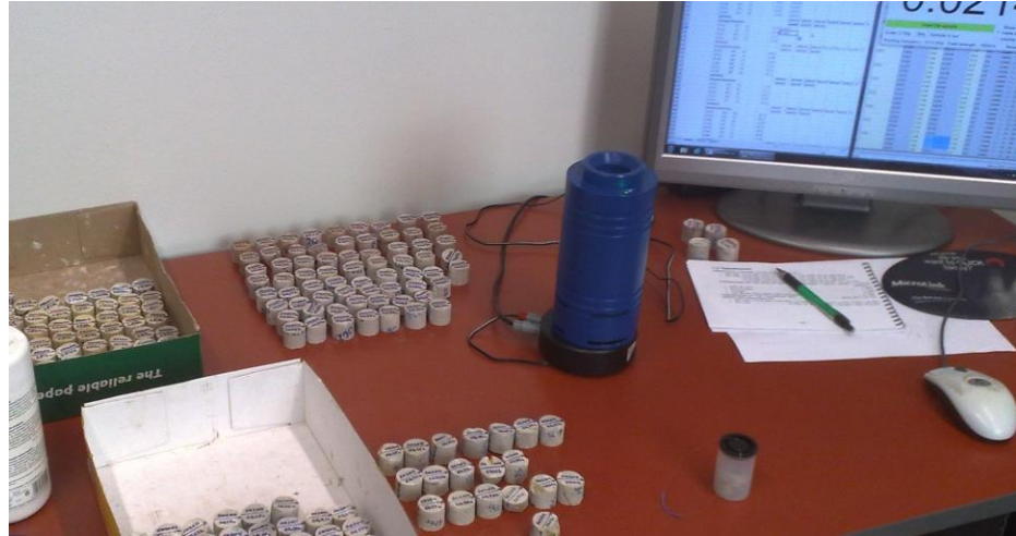
Figure 3. Magnetic susceptibility meter SM-100 with some of the specimens.
