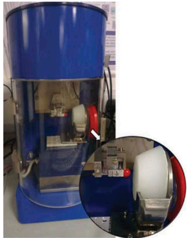
FIG. 2. MUST tester indenting sample stimulus with a hard tip.
