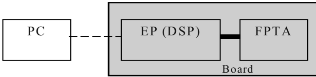
Fig. 2. Block diagram of our stand-alone board level evolvable system (SABLES)
