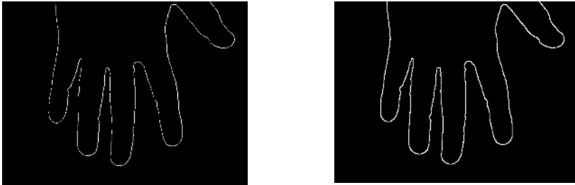
Fig. 6. Edges detected with Laplacian and Sobel filters in the hardware implementation.
