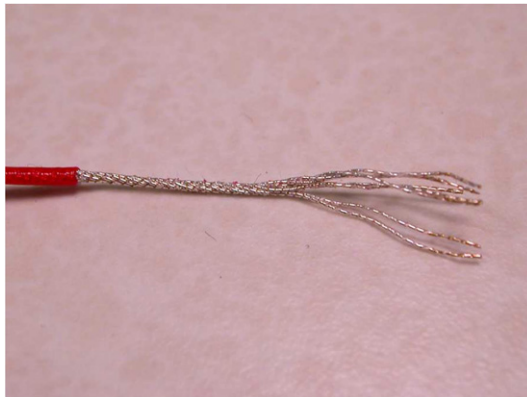
Fig. 5. Tinsel wire insulated with a detergent resistant coating.
