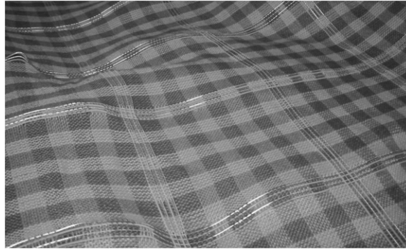
Fig. 15. A fabric with a fine-scale weave pattern with conductive fibers that allows for multiple placement points for components.
