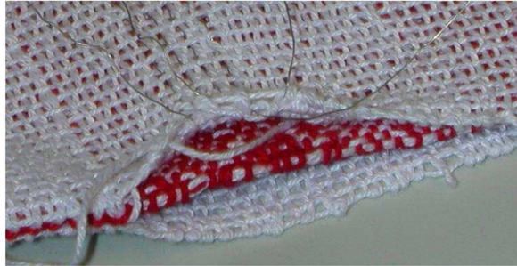
Fig. 2. An exposed view of the multi-layer fabric.
