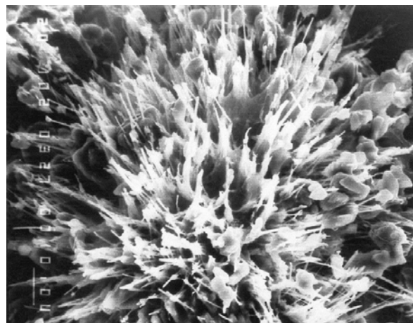
Fig. 1 Image of a specimen with an addition of CA – 26 days after the application of CA (at a depth of 50 mm into the concrete sample) [7]
