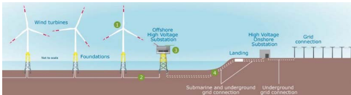
Fig. 1 Offshore wind farm main components [1]
