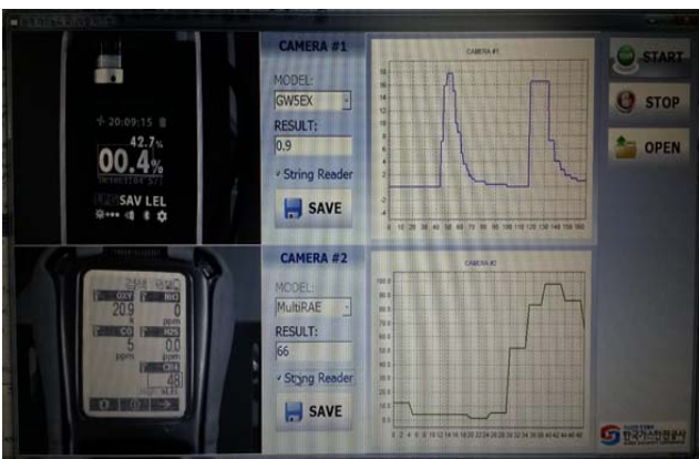
Fig. 12 Graphs of measured concentration for testing of two gas leakage detectors (175 seconds)
