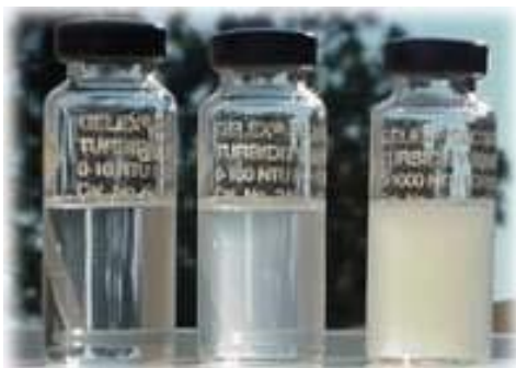
Gambar 2. Standar turbiditas 5, 50 dan 500 NTU (Wikipedia, Turbidity Available: https://en.wikipedia.org/wiki/Turbidity , diakses 28-10-2016)
