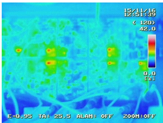
Fig. 5. Thermal field distribution on the PCB measured in a climatic chamber at 5 °C.
