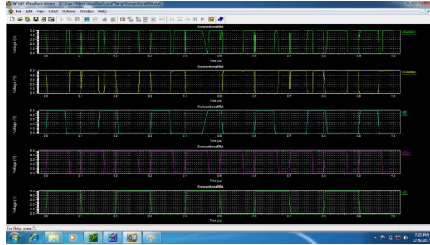
Fig.15.Output waveform for full adder
