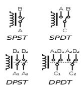
Fig.4 Circuit diagram of relays
