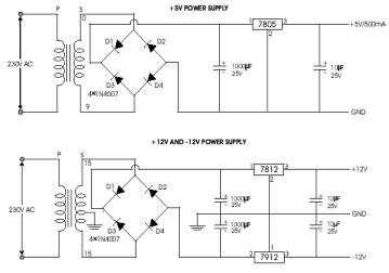
Fig. 2 Circuit Diagram of Power Supply
