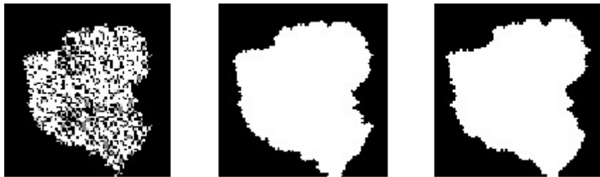
Fig. 2. Originally segmented image, dilated image, eroded image (from left to right).
