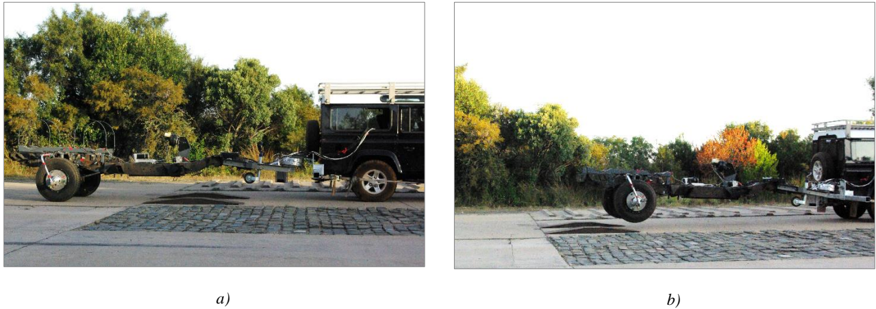
Fig. 4. ADAMS model validation over two symmetric ramps: a) 10 km/h b) 20 km/h
