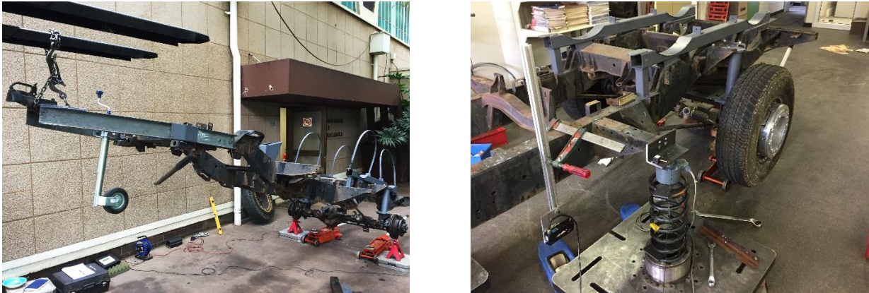
Fig. 2. Determination of center of gravity and Inertia for test trailer
