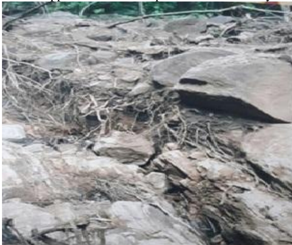
Fig 3a: The initiation of debris flow by the wedge failure at the crown of the scar
