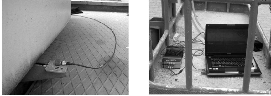
Fig. 8. Locations of the sensors on the foundation and basket
