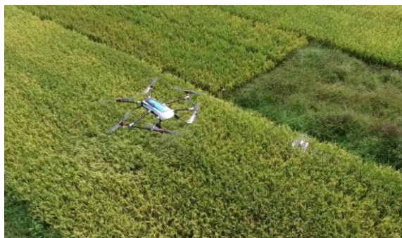
d. TXA-Xiangnong UAV spraying on rice by Guangzhou Tianxiang Aerospace Science and Technology Co., LTD
