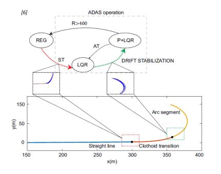
• **Concept:** Perform an aggressive drift manoeuvre to maximize the lateral acceleration.
