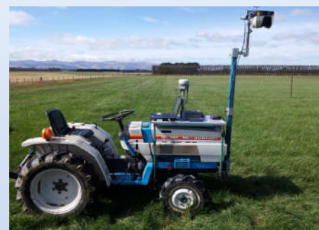
Tractor with LiDAR, GPS, and ruggedized laptop
