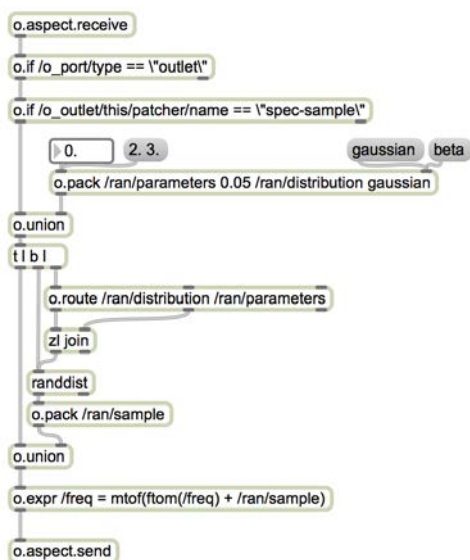
Figure 9: An aspect used to experiment with different probability distributions for smearing the spectrum.
