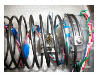
Figure 7. Measuring length variation with a joystick
