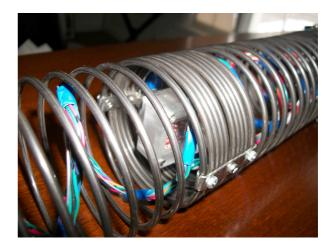
Figure 9. Accelerometer and gyro at coil's middle point
