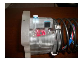
Fig. 4. LH unit: accelerometer, thumb and index switches
