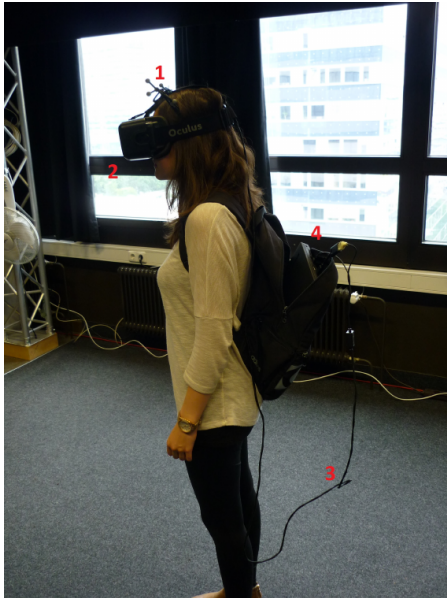
Figure 6: A fully equipped test person with tracking system target (1) and Oculus Rift (2) connected via cable (3) to the control laptop (4).
