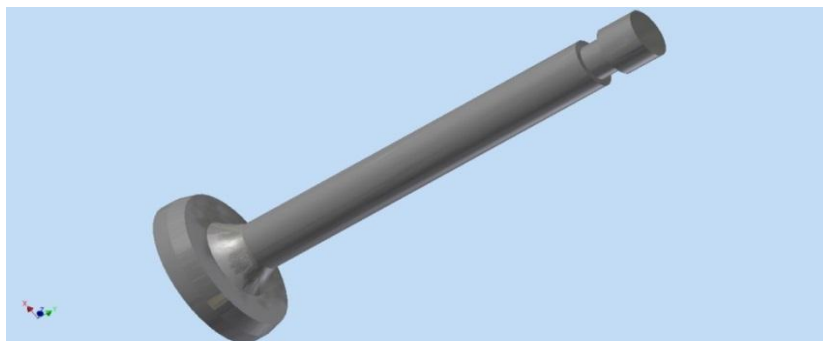
Figure 10: 3D Modelling of poppet valve
