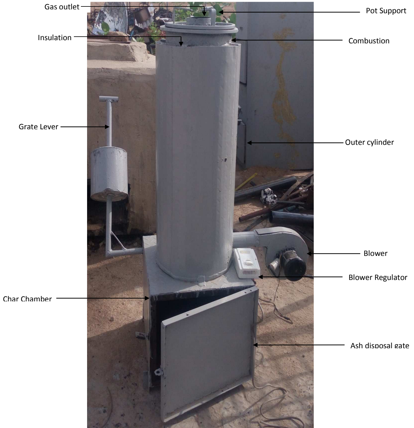
Figure 3: Constructed biomass gasifier stove
