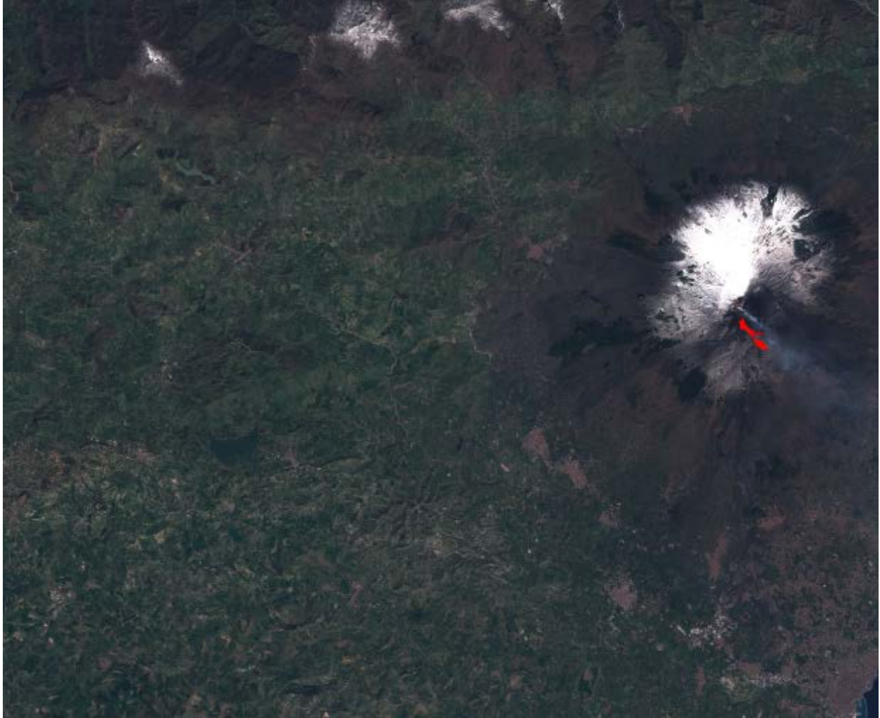
Figure 3: NOVELTIS systematic processing service VEGAN HSP created this Hot Spot Map based on a Sentinel-2 acquisition of the 19 th of March 2017. The lava flow of Mount Etna is visible in bright red on the right side of the image.
